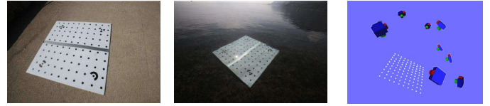
Figure 4a,b,c: Raw calibration images in air(a) and two media (b) and camera positions(c).
